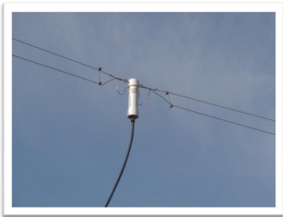
Photo #1 Center Insulator
