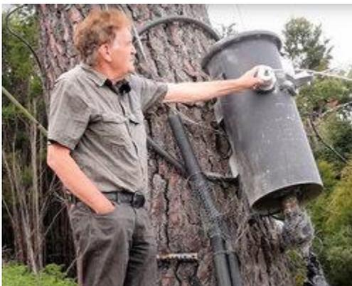
Watson said he made the 600 W ladder line himself and he uses the antenna on all bands, typically running only 200 W. The coaxial feed line goes to his house down a slope from the antenna via a conduit. His home is entirely off the grid, powered by solar power. The noise level is very low at his location, with power lines some distance away, although his solar power system's inverter is nearby.
