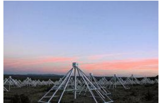
The Long Wavelength Array at Sevilleta National Wildlife Refuge is capable of imaging the entire sky at once, allowing AFRL scientists to track and characterize sporadic E. The facility consists of 256 dual-polarization dipoles. [Ken Obenberger, photo]
